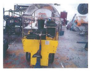
The bucket at the front is sitting proud in this photo. It will be lower, in line with the others when in use. There will also be a rear view mirror on the tricycle. The seat on the tricycle will be higher when in use to give the rider better all-around vision.
